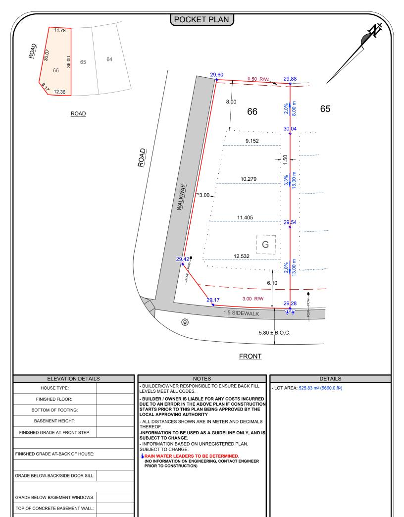
LEGEND DESIGN GRADE ELEVATION PROPOSED CLEAN OUT PROPOSED HYDRANT PROPOSED BACK OF CURB B.O.C PROPOSED STREET LIGHT (3) PROPOSED BACK OF WALK B.O.W AS-BUILT ELEVATION PROPOSED SERVICE PEDESTAL 000 PROPOSED C.C. LOCATION PROPOSED POWER SERVICE PROPOSED LIP OF LANE L.O.L PROPOSED ELEVATION 00.00 PROPOSED TRANSFORMER CENTERLINE ELEVATION ٧
